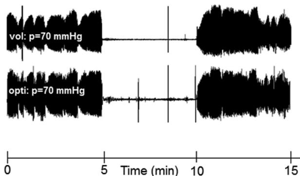
**Fig. 5.** Simultaneous recordings of PAT volumetric and photoplethysmographic signals from the same tissue bed, over 15 min. Both signals recorded within the same PAT probe on the same finger. Note a 5 min period of arterial occlusion between 5 and 10 min.
